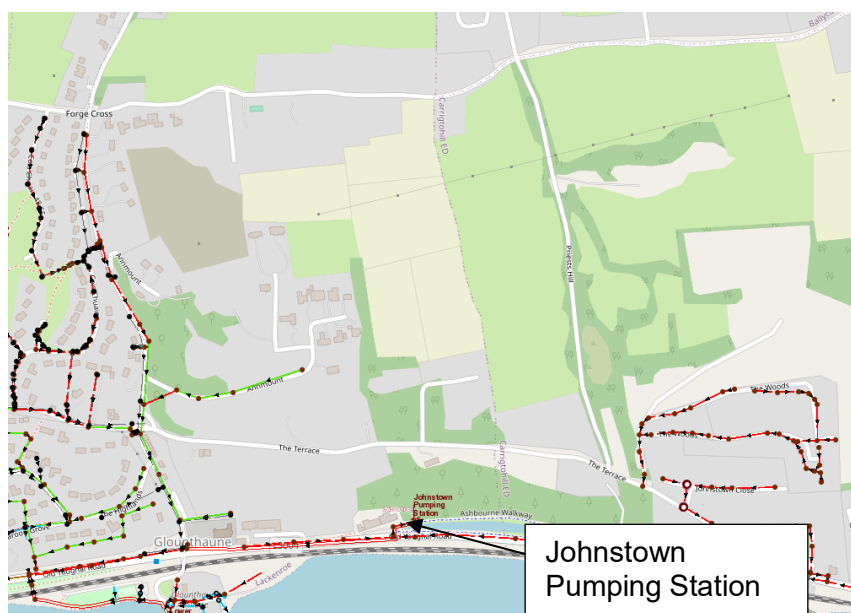
Figure 3-2 – Existing Wastewater Drainage Network
